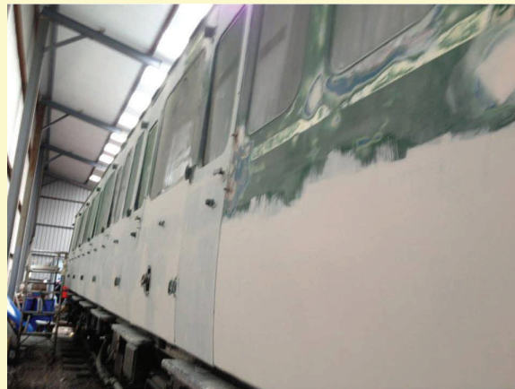
Bodywork & repaint progression on M55006 - anyone for white & blue stripe!??
